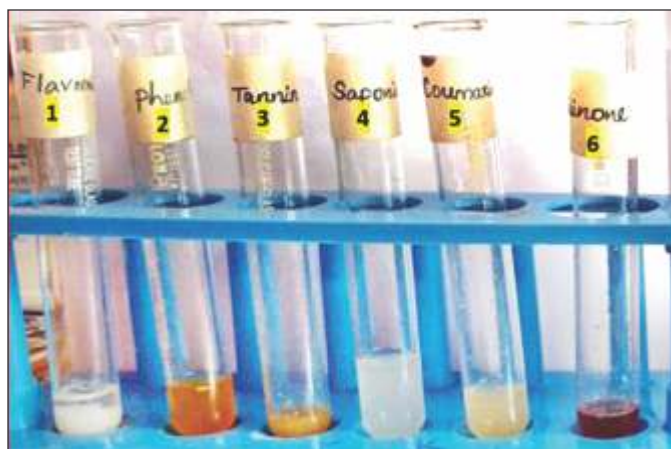
Fig. 1. Results of qualitative analysis of Aqueous and Ethanolic Tridax procumbens leaves, showcasing positive and negative outcomes. 1. Shinoda test (Flavonoids), 2. FeCl 3 test (Phenol), 3. Lead acetate test (Tannin), 4. Foam test (Saponin), 5. Sodium chloride test (Coumarins), 6. KOH test (Quinine)
